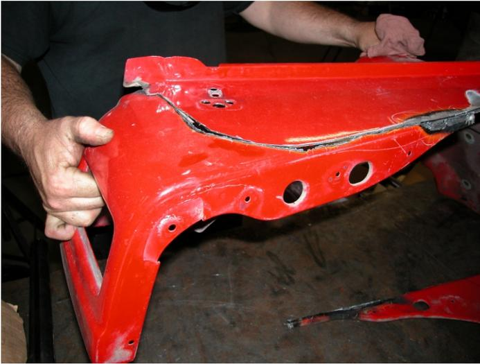
1. Remove the front fender from the vehicle completely. This means both right and left sides. On the passenger side, this will require removal of the battery from the Jeep. After removing front fenders, remove material as shown. Use an abrasive cut-off wheel, or plasma cutter.
