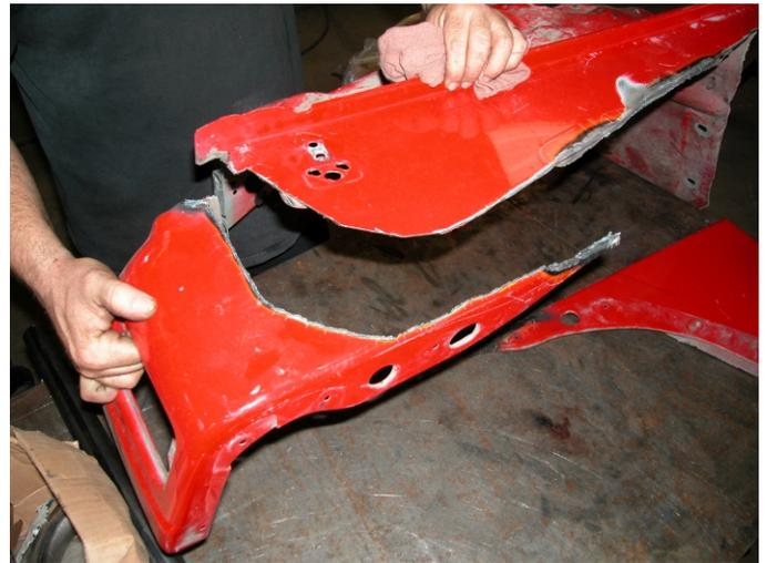
3. Remove the entire lower rear section as shown. Cut vertically down the inner side of the wheel well and remove all of the outside face of the fender.
